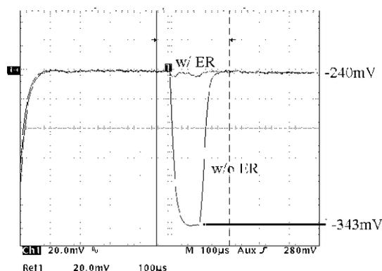
Figure 2: Energy recovery with a 100 $\mu$ sec beam pulse: Response of the rf forward power signal with (-240mV) and without (-343mV) energy recovery
