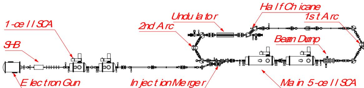
Figure 1: Layout of the JAERI energy-recovery linac
