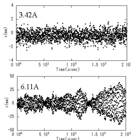
Figure 3: Bunch position vs. time for 3.42A beam current, approximately threshold (top), and for 6.11A beam current, above threshold (bottom)
