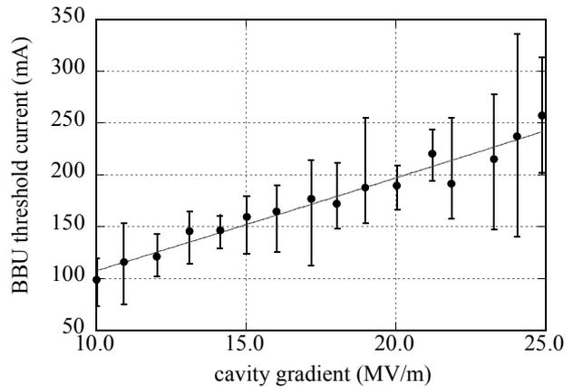
Fig. 5: BBU threshold current vs. cavity gradient.
