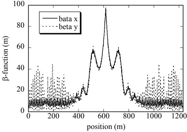
Fig. 2:  $\beta$ -function in the linac as a result of the optimization.
