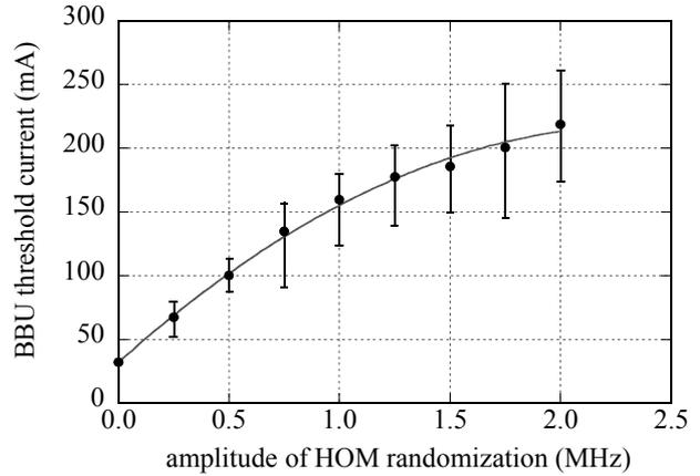
Fig. 4: BBU threshold current vs. amplitude of HOM randomization.
