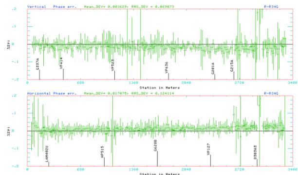
Figure 8. Measured horizontal and vertical plane phase advance error with the medium beta straight in place.
