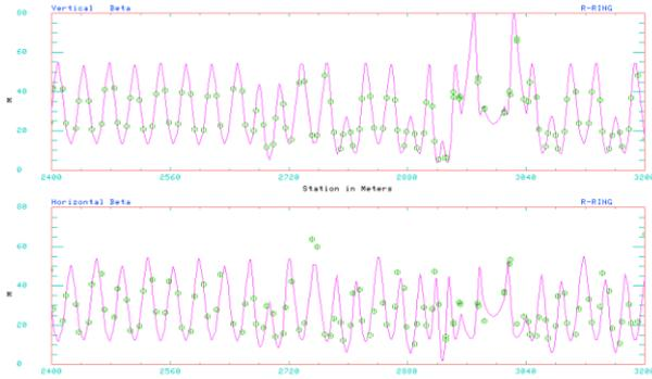
Figure 9. Measured horizontal and vertical beta functions compared with model calculations over a stretch of 800 m, including the medium beta straight region.
