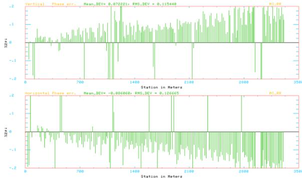
Figure 4. The phase advance errors as measured before the end-shim replacement using first turn orbit data. The cumulated phase advance error is about +0.15 in the vertical plane (top plot) and 0.18 for horizontal plane, in units of  $2\pi$ .
