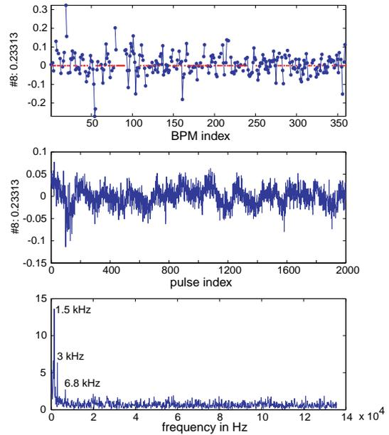
Figure 6: The eighth mode is unrelated to the horizontal kick. Its spectrum shows peaks around 0.36, 1.5, 3, and 6.8 kHz. The zig-zag motion suggests that it may be due to feedback. In fact, some of these frequencies are connected with the real-time feedback system. Power line noise could be a factor as well.
