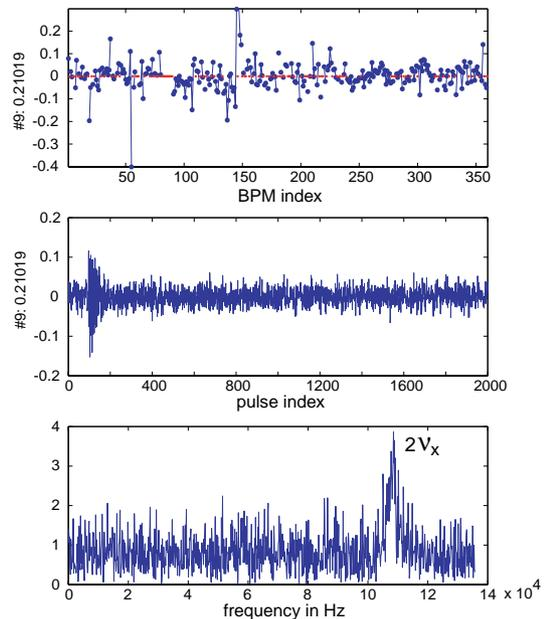
Figure 7: The ninth mode oscillates at  $2\nu_x$  indicating non-linear effects due to either lattice or BPM nonlinearity. The spatial vector suggests large effects around BPM 50 and 150. It is remarkable that the spatial-temporal mode analysis can clearly resolve this mode even at such a low signal level.
