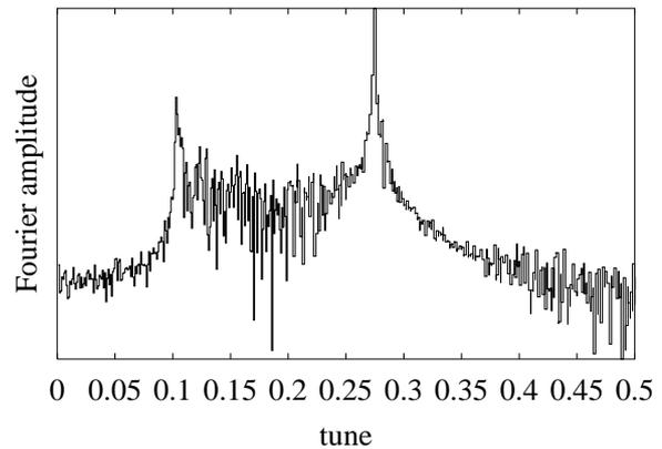
Figure 3: Fourier spectrum of the transverse dipole signal at  $\xi = 0.17$  (logarithmic scale).
