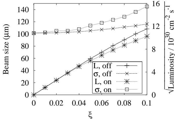
Figure 4: Beam size at IP and square root of the luminosity vs. the beam-beam parameter. Comparison of the sextupoles on and off options,  $\beta^*=6.3$  cm.
