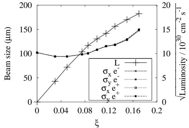
Figure 2: Beam size at IP and square root of the luminosity per 1 IP vs. the nominal beam-beam parameter. Linear machine optics.
