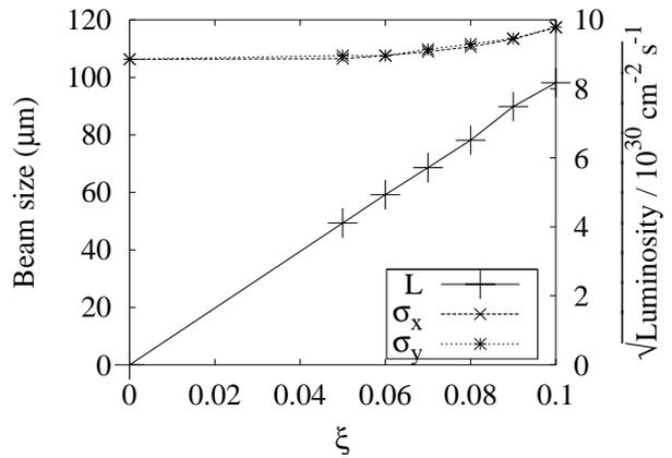
Figure 6: Beam size at IP and square root of the luminosity vs. the beam-beam parameter,  $\beta^*=10$  cm.
