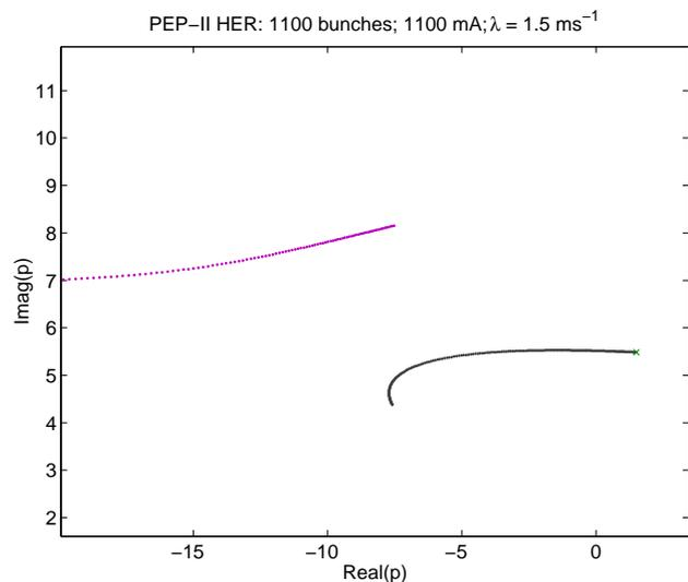
Figure 4: Gain locus study for a proposed woofer filter for the PEP-II HER. The unstable growth rate without feedback is  $1.5 \text{ ms}^{-1}$  at 1100 mA. Increasing the woofer gain to the 44 dB of Figure 3 produces damping rates of  $-4 \text{ ms}^{-1}$ .
