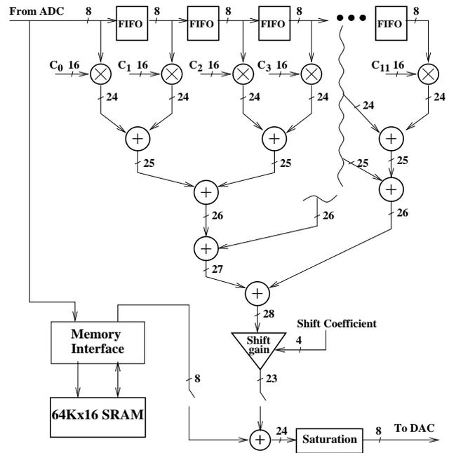
Figure 2: Block Diagram of the EPLD implemented 12 tap FIR filter. The figure explicitly shows 5 taps; the structure of the adder tree is shown where it is extended for the 12 tap filter, with 12 coefficients and multipliers. Also shown is a diagnostic memory used for transient domain measurements.
