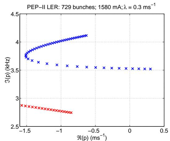
Figure 1: Gain-locus plot showing the maximum damping possible through the woofer in the PEP-II LER. With no gain the instability growth rate for the most unstable mode is  $0.3 \text{ ms}^{-1}$ . With increasing woofer gain a maximum damping of  $-1.5 \text{ ms}^{-1}$  is reached. Increasing the channel gain beyond this point simply produces greater reactive tune shift, as well as less resistive damping.
