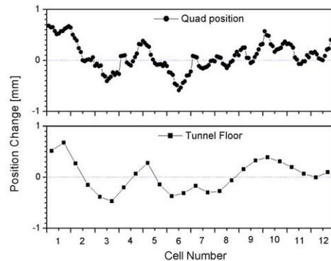
Figure 4: The vertical position change from February to July 2002; upper figure: quadrupole magnets, lower figure: SR tunnel floor elevation.
