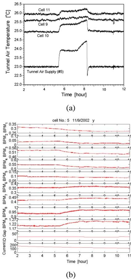
Figure 1: The tunnel air temperature at cell 9, 10, 11 (a) and BPMs in the vertical plane at cell 5 (b) when the supply air temperature for those cells increases rapidly about  $1^\circ\text{C}$  for 3 hours. The unit of BPMs in (b) is mm.
