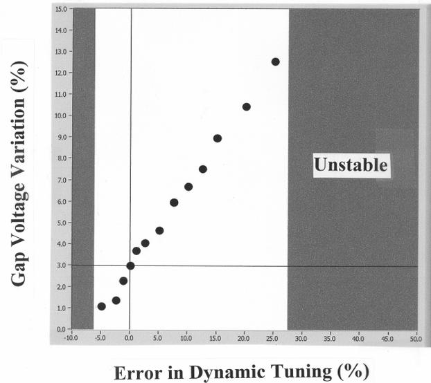
Figure 3. Buncher-cavity gap-voltage variation over SNS beam cycle due to errors in time dependence of the dynamic tuning analogue of the Smith compensator.
