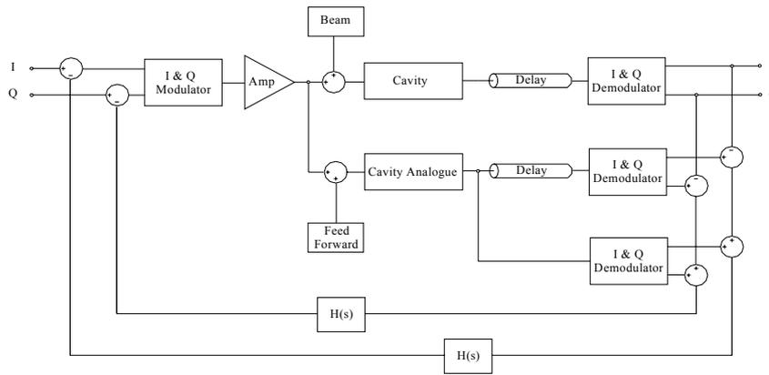
Figure 1. Ring RF Feedback System Utilizing Smith Corporation
