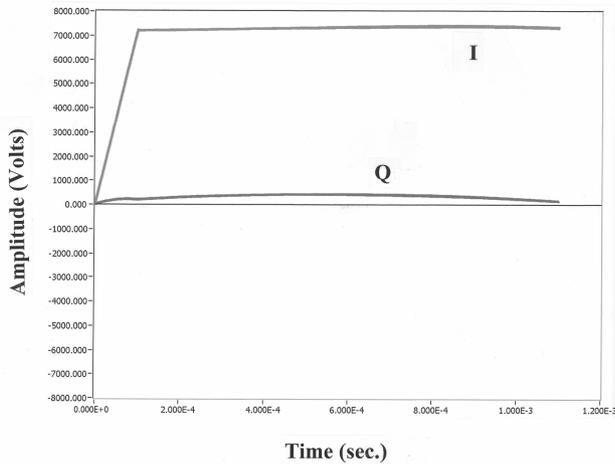
Figure 2. In-phase, I, and quadrature, Q, components of gap voltage with Smith compensation at full beam current.
