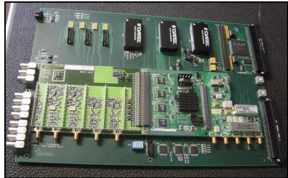
Figure 4. The prototype Field Control Module. The Analog Front End, Digital Front End, and RF Output daughtercards (left to right) are mounted on the VXI motherboard.
