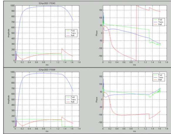
Figure 7. Demonstration of effect of piezoelectric tuner on dynamic cavity performance. Open loop operation at 12.5 MV/m for two cases: piezo tuner inactive, and piezo tuner driven with rectangular pulse having width=860  $\mu$ s, amplitude=220 V, and lead=580  $\mu$ s.
