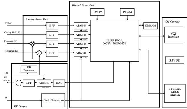
Figure 1: FCM Block Diagram
