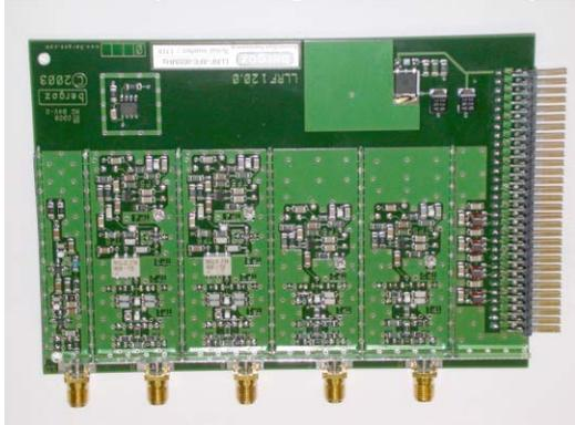
Figure 2: LLRF Analog Front End daughter board from Bergoz Instrumentation.
