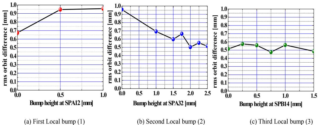
Figure 5: Rms orbit difference between first and second bunches versus bump height. The rms orbit difference calculated from the all BPMs between SPA12 (first bump position) to SPR01 (entrance of J-arc section). Three local bumps were contracted successively. In the case of (c), therefore, three local bumps were simultaneously constructed.
