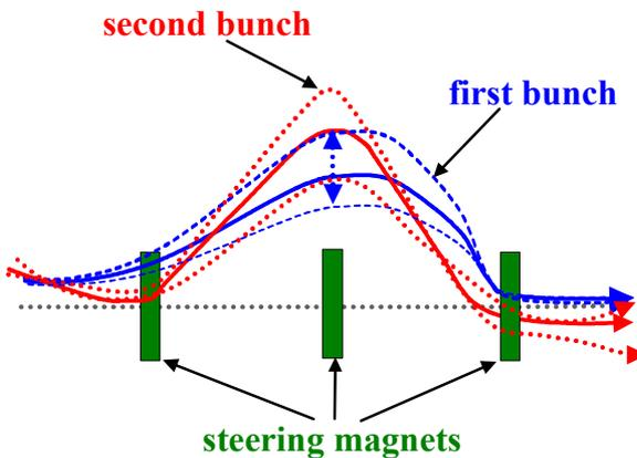
Figure 3: Schematic drawing of a new two-bunch orbit correction method using the transverse wake field kick caused by first bunch.
