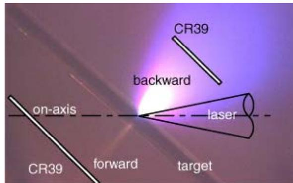
Figure 1: Picture of the interaction between the laser with intensity of  $\sim 4 \times 10^{16} \text{ W cm}^{-2}$  and  $3 \mu\text{m}$ -thick Al target foil with schematic of the experimental setup. Definitions of “backward” and “forward” sides are also given.
