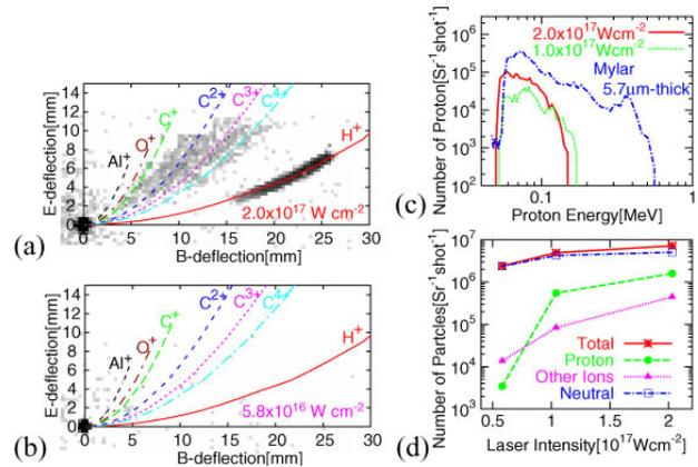
Figure 3: (a) and (b) Thomson parabola spectra from Al 3  $\mu\text{m}$ -thick targets in the forward direction. (c) Proton spectra obtained at laser intensities above  $10^{17} \text{ W cm}^{-2}$  from the Al targets. A dot-dash line shows the case of mylar in 5.7  $\mu\text{m}$ -thick with  $2.1 \times 10^{17} \text{ W cm}^{-2}$  laser intensity. (d) Dependence of the number of particles on the laser intensity.
