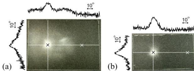
Figure 2: Typical CR39 images of generated particles in the forward direction. Target was Al in 3  $\mu\text{m}$ -thick. Black cross indicates the direction normal to the target surface and white cross indicates on-axis direction. Curves show distributions of etch pits along the path indicated in white lines. Laser intensities were (a):  $2.1 \times 10^{17} \text{ W cm}^{-2}$  and (b):  $1.1 \times 10^{17} \text{ W cm}^{-2}$ .
