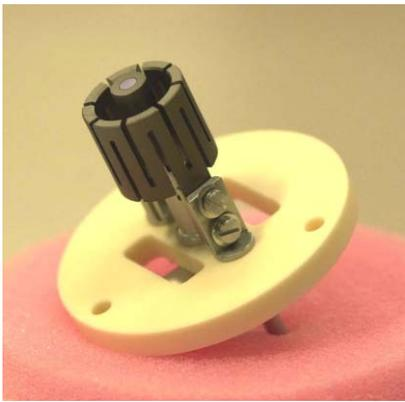
Figure 2: CeB<sub>6</sub> cathode assembly
