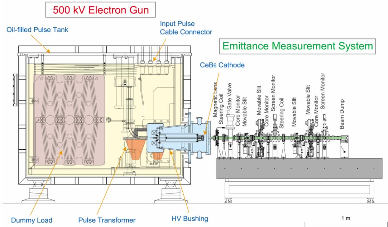
Figure 6: 500 kV Electron Gun Test Stand
