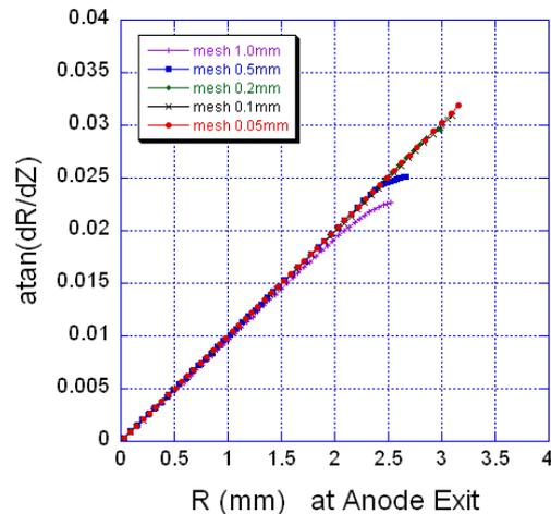
Figure 5: Phase space plot for various mesh sizes
