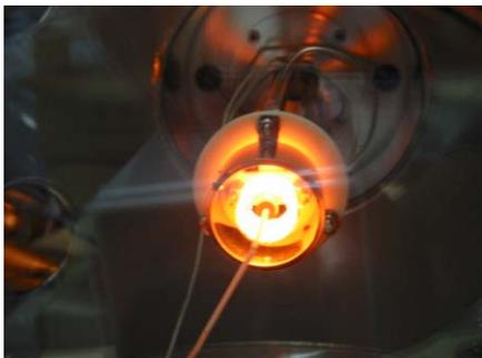
Figure 3: Heating test for the graphite heater
