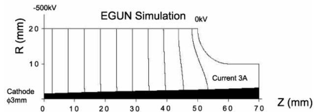
Figure 4: Beam trajectory simulated by the EGUN code
