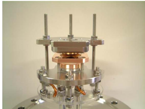
Figure 2: Triode gun with adjustable electrodes
