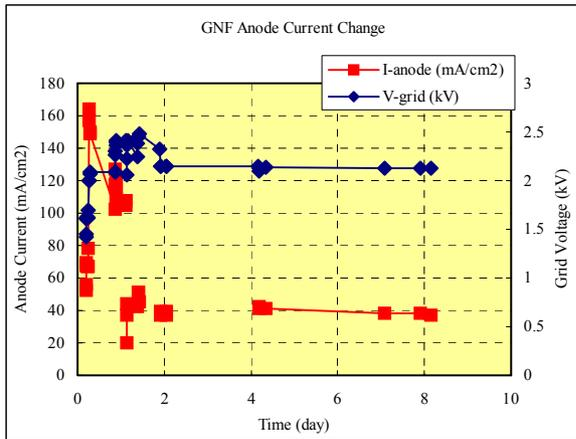
Figure 5: Characteristics of GNF
