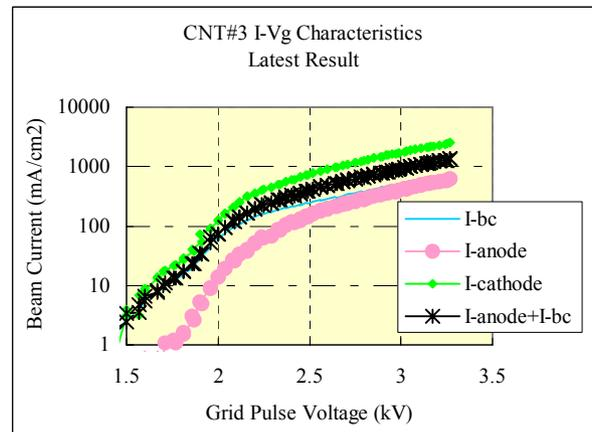
Figure 5: CNT#3, 2<sup>nd</sup> Grid voltage vs. Emission current.
