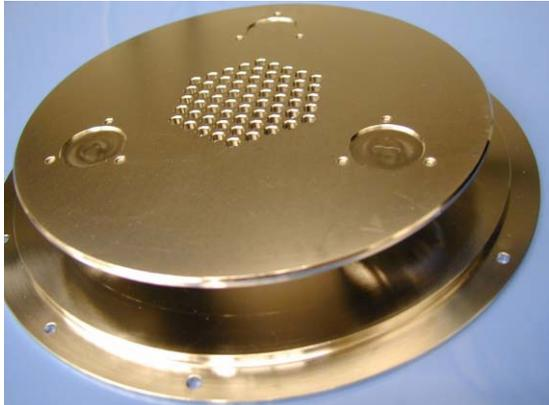
Fig. 7: Extraction plate for the 61-beamlet array.
