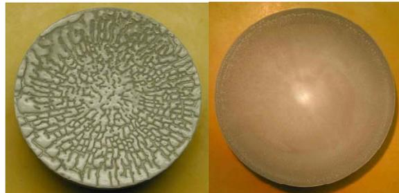
Figure 3: Comparison of significant coating technique improvements fabricating 10cm diameter, 0.4mm K<sup>+</sup> alumino-silicate coatings on porous tungsten substrates.
