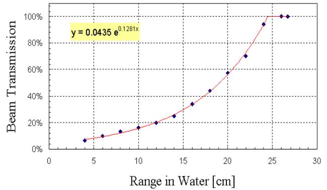
Figure 3. Transmission through ES1 vs. range in water.
