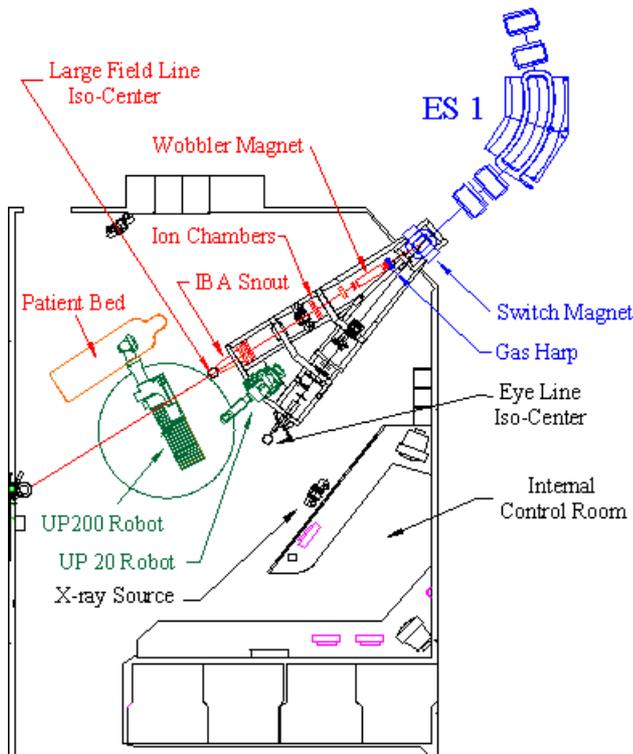
Figure 5. Layout of the fixed horizontal Treatment Room.
