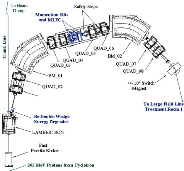
Figure 2. Layout of Energy Selection Beam line (ES1)
