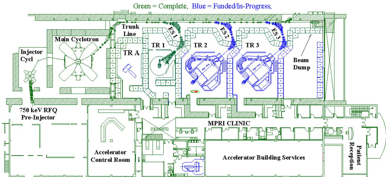
Figure 1. The MPRI Facility showing the IUCF cyclotrons, Trunk and ES lines, Treatment Rooms and Clinical Facilities.
