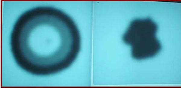
Figure 6: Radiographic film showing beam scanning. The left image is a raster scanned beam using intensity modulation to achieve the varying intensities. The right image only uses beam on and off states.
