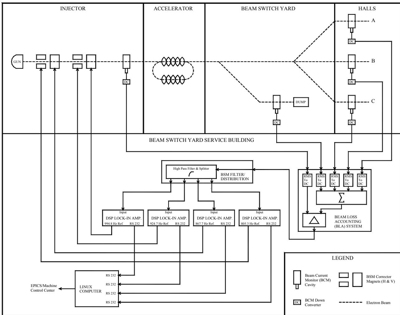
Figure 1: Block diagram of BSM system.
