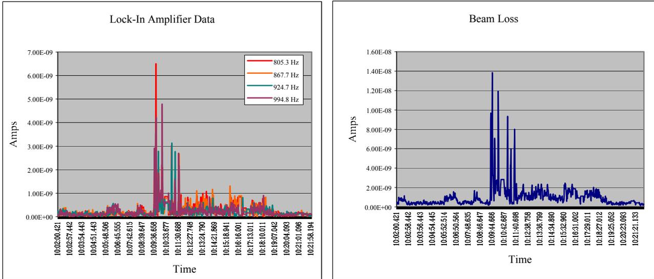
Figure 2: Data from the four lock-in amplifiers and corresponding beam loss.
