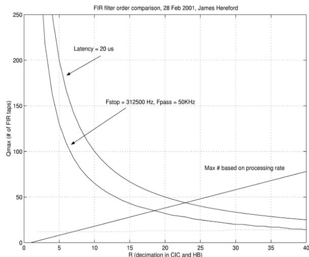
Figure 1: Decimation, R, vs number of FIR taps (Q). 20 $\mu$ s latency contour added for reference.
