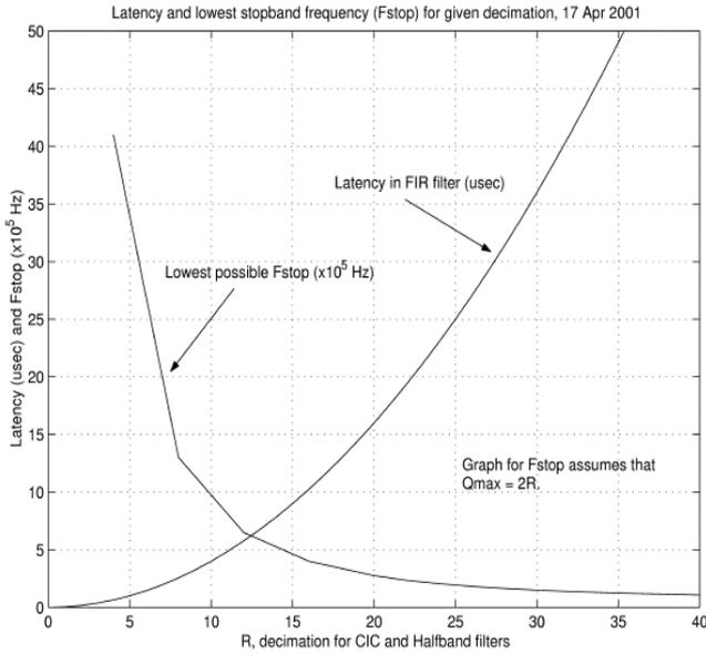
Figure 2: Decimation, R, vs Latency and stop-bandwidth,  $F_{stop}$ .
