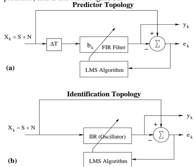
Figure 3: Adaptive prediction topology is shown at (a).  $X_k$  is input signal plus noise, while predicted and error signals are  $Y_k$  and  $e_k$ , respectively. FIR coefficients are denoted by  $b_k$ . Adaptive Identification is shown in (b).
