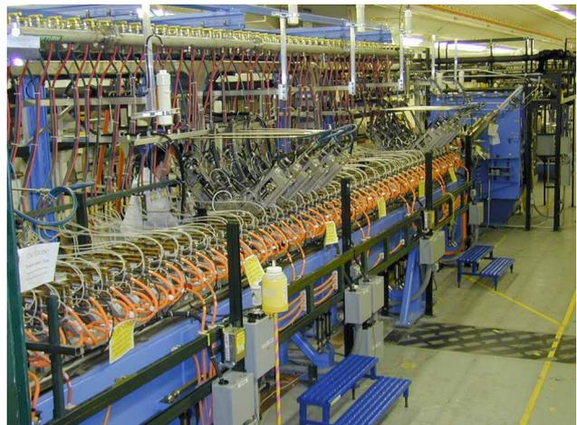
Figure 1. Shown above is the 52 quadrupole magnet lattice with the two clusters of WS/HS beam profile measurements.
