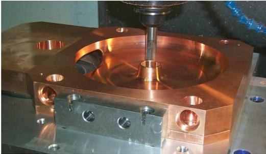
Figure 3. Machining tuning ring on finished end cell.
