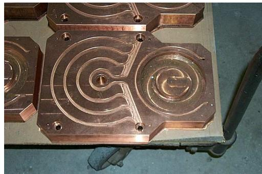
Figure 2. Completed half-cell septum
