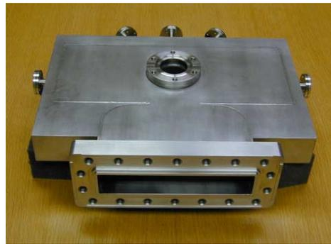
Figure 6 Photograph of L-band gun cavity
