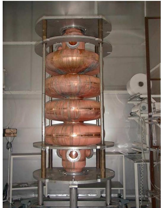
Figure 7: Prototype cavity optimized for  $\beta = 0.7$ .
