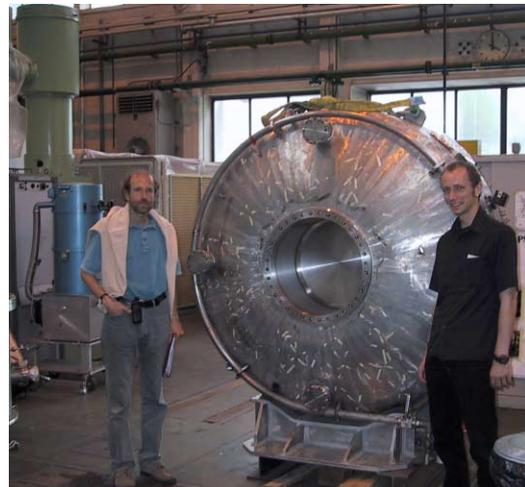
Figure 6: CERN 88 MHz test cavity.
