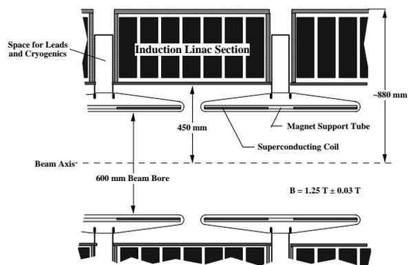
Figure 3: Cross section through induction linac cell.
