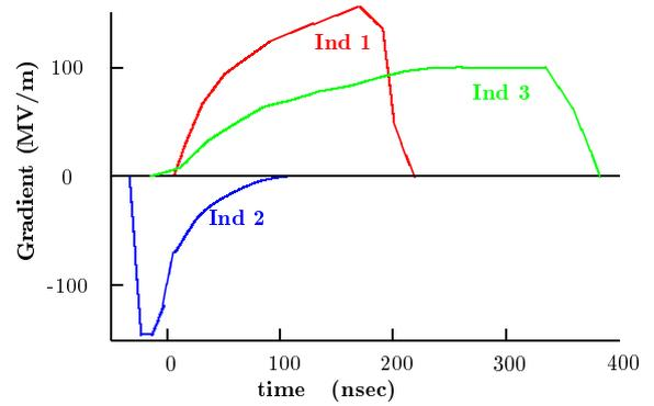
Figure 4: Acceleration waveforms for induction linacs 1, 2 and 3
