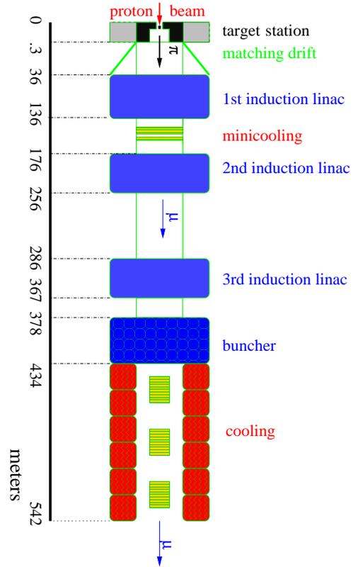
Figure 1: Layout of the front end of a Neutrino Factory
