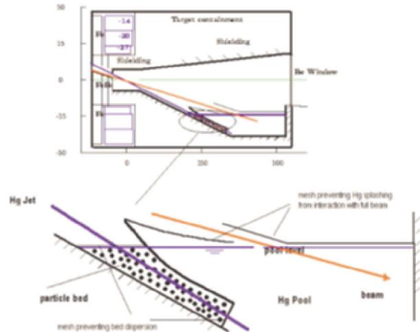
Figure 4: A mercury pool inside the capture solenoid intercepts the mercury jet and the unscattered proton beam.
