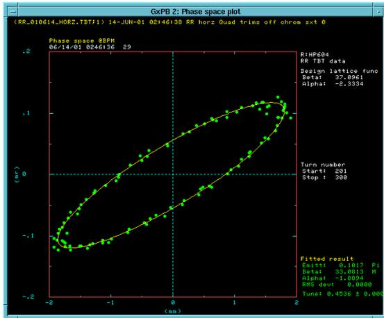
Figure 1: Turn-by-turn beta function measurement
