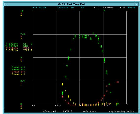
Figure 3: Aperture scan using three-bump, DCCT and BLM's
