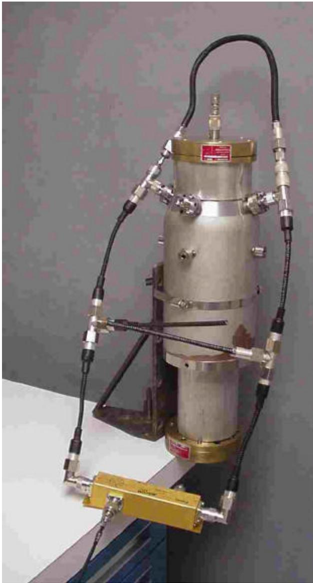
Figure 5 – Photo of stub tuned resonant BPM showing testing configuration. Matching sections at each end carry a RF signal through a center conductor to a termination. Output is taken from the difference port of a Hybrid transformer.
