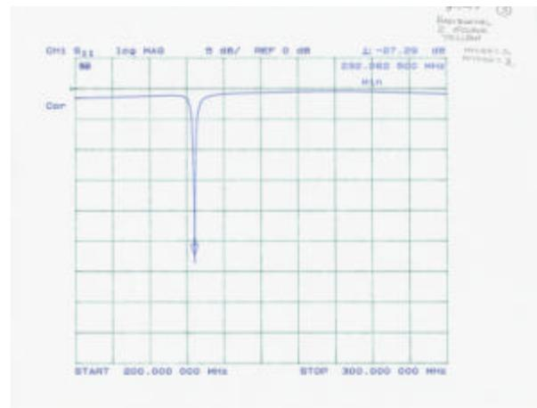
Figure 6 - Reflection coefficient for the Horizontal Plane Hybrid Difference port, Movable BPM located at 2 O'clock on the Yellow beam line
