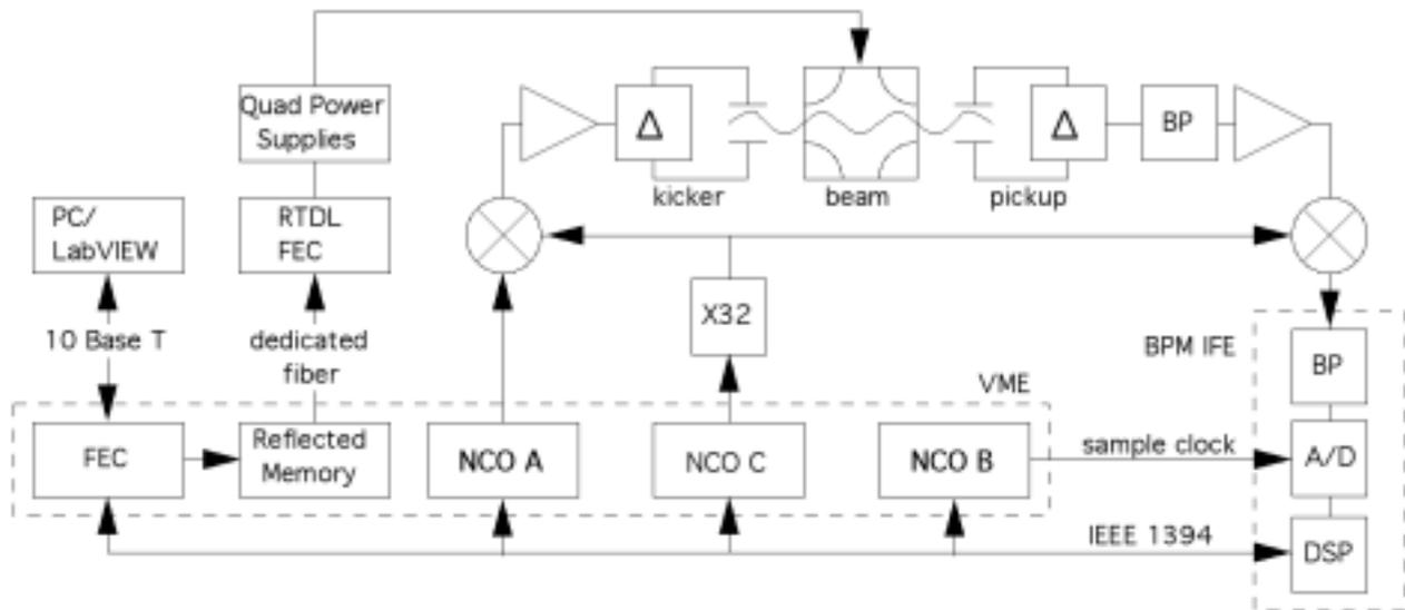
The digitizer clock is generated by NCO B at 4x the frequency of NCO A (or 312KHz), permitting a simple I/Q demodulation[8] of the signal. The data is processed in the DSP of a modified RHIC BPM module[9]. The following functions are performed by the DSP:
