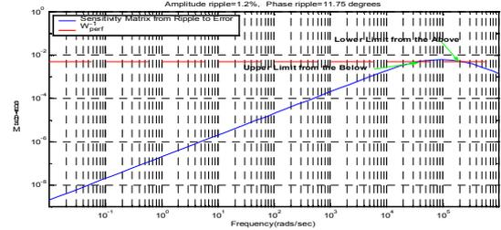
Figure 2: Transfer Matrix from the scaled High Voltage Power Supply (HVPS) ripple to the tracking.
