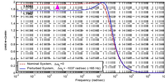
Figure 3: Maximum singular value plot of the open loop nominal system and the open loop perturbed system for a SRF cavity.
