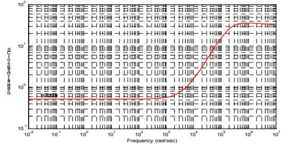
Figure 4: Maximum singular value plot of the scaling transfer matrix  $C(s)S(s)$ :  $C(s)$  is the transfer matrix of the PI feedback controller and  $S(s)$  is the sensitivity matrix.
