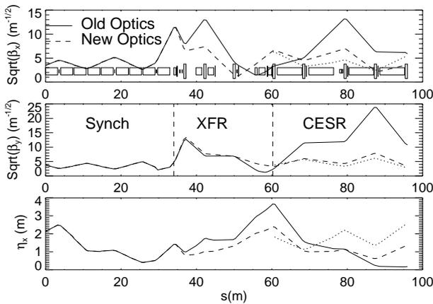
Figure 1: Extracted electron beam optics. The dotted line shows the CESR stored beam optics (starting at 60m). The old (unmatched) optics are compared to the new (matched) optics.
