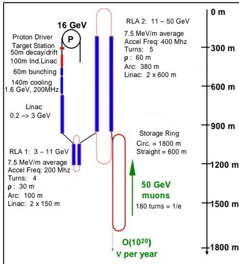
Figure 4: Footprint of a 50 GeV Facility.
