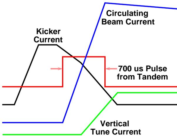
Figure 2: Typical Timing at Booster Injection.
