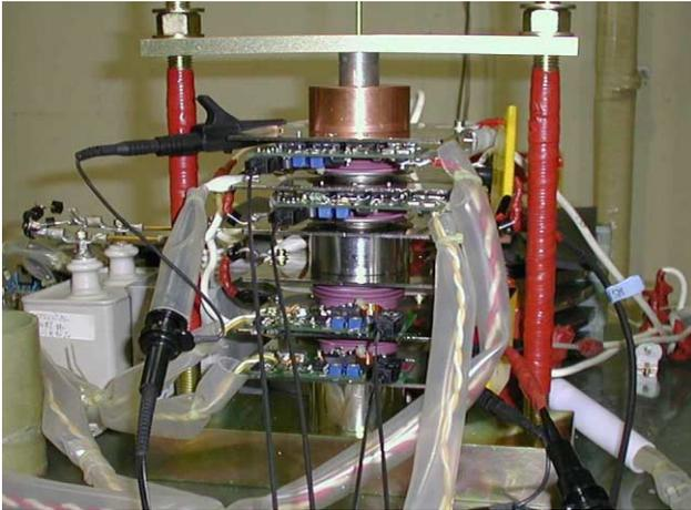
Figure 2: Test stand of modulator assembly.
