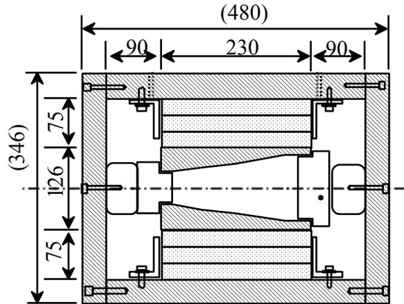
Figure 4: Cross-section of a prototype magnet.
