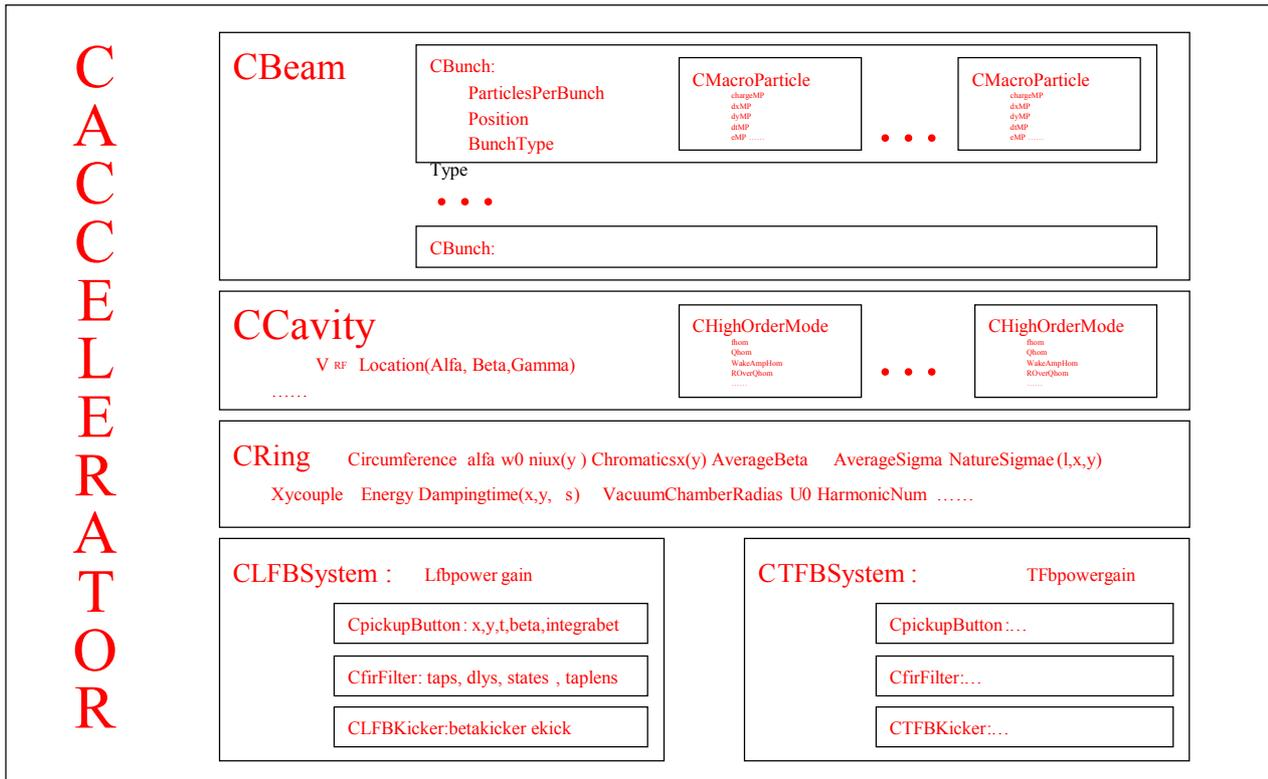
Figure 1 Classes description of an accelerator
