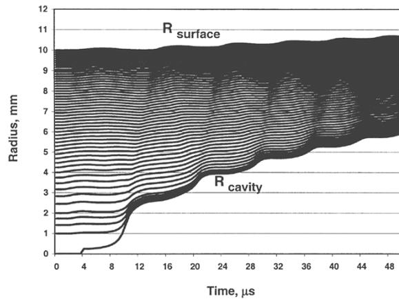
Fig. 2. Dynamics of cavity growth in Hg target
