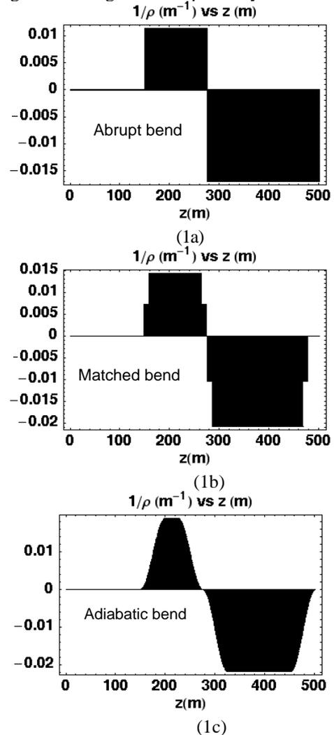
Figure 1. Inverse instantaneous radius of curvature ( $m^{-1}$ ) as a function axial distance (m) for (a) an abrupt bend, (b) a matched bend, and (c) an adiabatic bend, using
