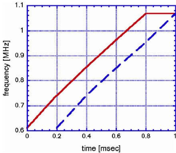
Figure 5: The rf function of the two bunch acceleration. In the POP FFAG, We kept the frequency separation of 100kHz .
