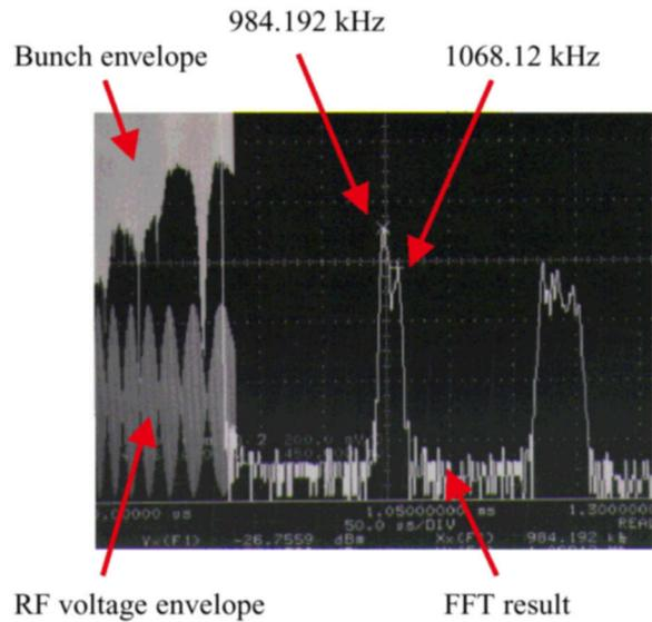
Figure 6: Observed beam signal. There are two frequency peaks on the beam signal after two bunch acceleration.
