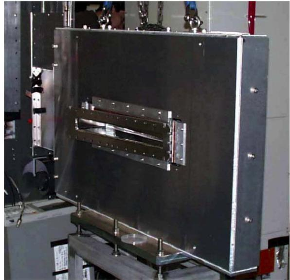
Figure 1: The rf cavity using two rectangular 'FINEMET' cores of 1.1m(width) x 0.7m(height).
