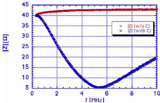
Figure 2: The frequency characteristic of the matching transformer as a function of the frequency.
