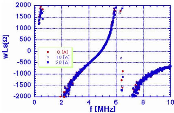
Figure 3: The choke inductance which supposed to be more than 1mH. The series resonance frequency was about 5.0MHz.
