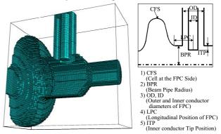
Figure 3. MAFIA 3-D model for the  $Q_{ext}$  analysis and the five parameters that affect  $Q_{ext}$
