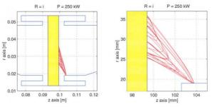
Figure 6: Multipacting trajectories between the window and the matching choke.
