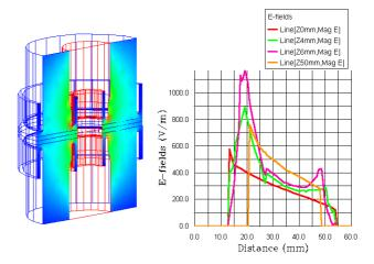
Figure 1: Half structure of 3-D model for the coaxial section of the ceramic window used in HFSS. Timeinstantaneous peak fields normalized to 1W input are shown near the ceramic window at z = 0, 4, 6, 50mm.
