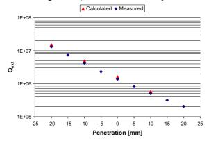
Figure 5:  $Q_{ext}$  calculated and measured for the  $\beta$ =0.61 cavity.
