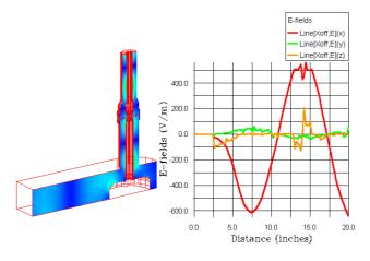
Figure 2: Half structure used in the HFSS modeling: the doorknob transition is integrated with the coaxial window.
