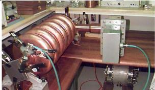
Figure 4: Q<sub>ext</sub> measurements setup.
