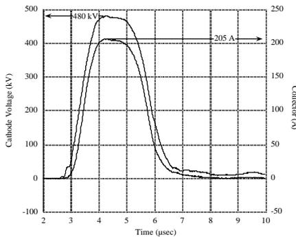
Figure 7. Measured gun voltage and current pulses.
