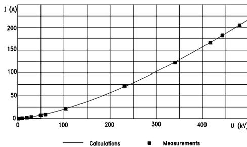
Figure 8. Beam current versus voltage.
