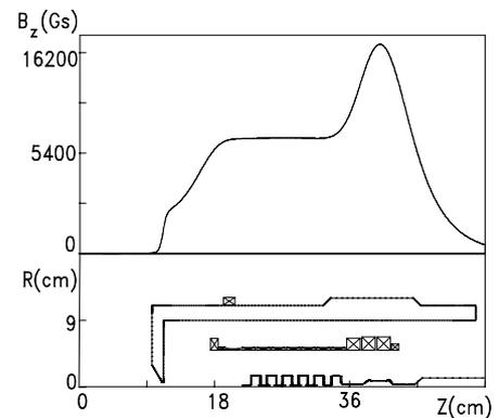
Figure 1. Magnetic system layout and magnetic field profile.
