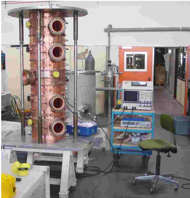
Figure 3: 500 MHz cavity piled up for frequency and field profile tuning
