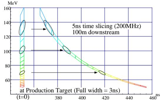
Fig. 1 Muon energy as a function of TOF at 100m from the production target.
