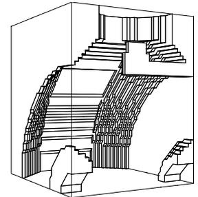
Fig. 6 Dual Frequency Cavity. The extra resonator splits the resonant frequency.
