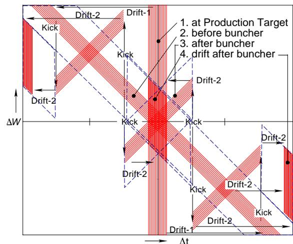
Fig. 2 Bunching scheme with large energy spread. Broken lines show an extreme case for the wide initial time spread.
