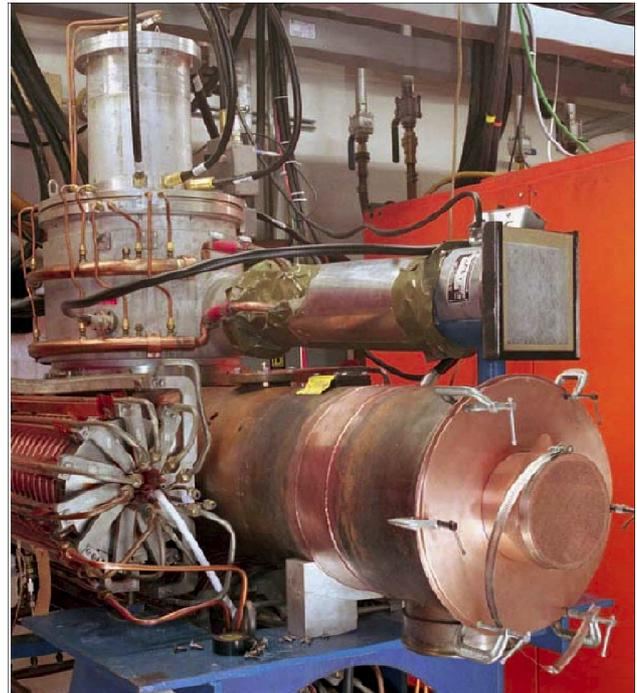
Figure 5. Photograph of the prototype large-aperture cavity with power amplifier at the test stand.
