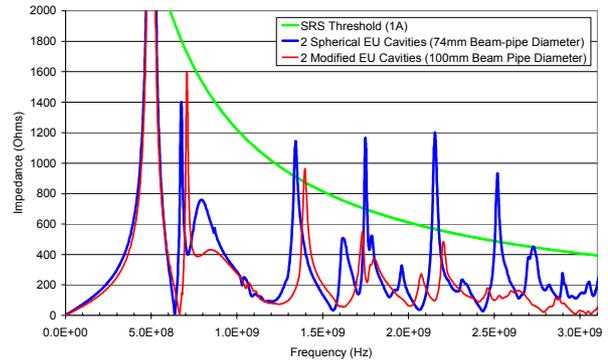
Figure 3. Cavity Longitudinal HOM Spectrum.
