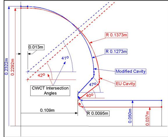
Figure 2. EU Cavity and Modified Cavity Geometries.
