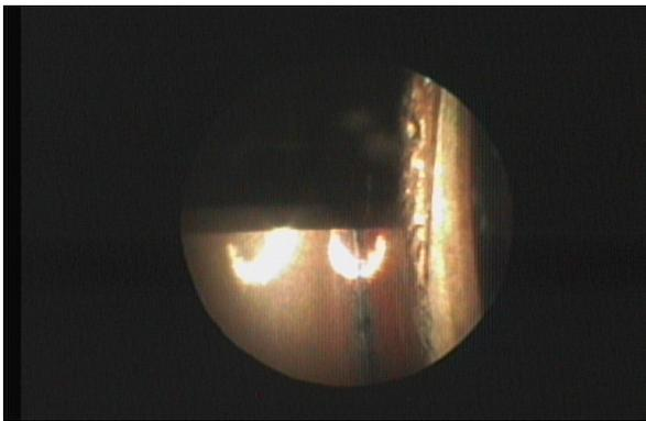
Figure 3: Damaged coupler iris, looking from the beam axis towards the coupling aperture. The section continues to the right.
