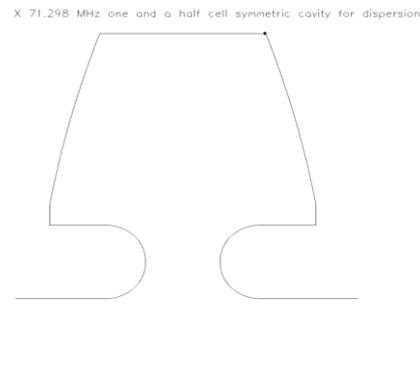
Figure 4. 71.26 MHz cavity with domed sides for mechanical strength.
