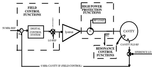
Figure 1: RF Control System block diagram.
