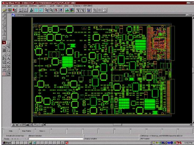
Figure 3: Motherboard PCB layout
