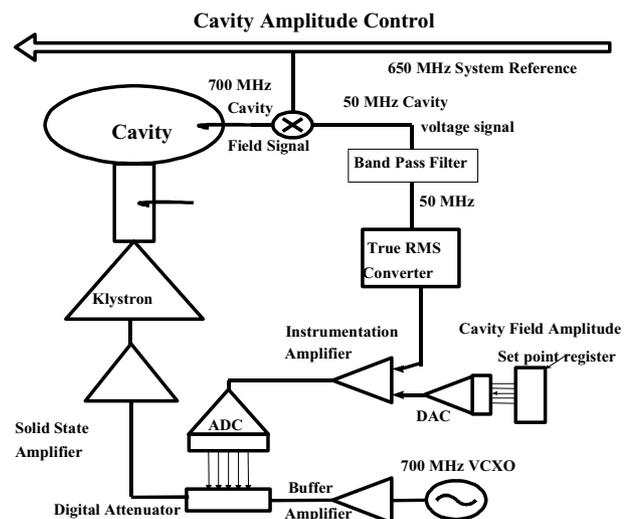
Figure 1. Cavity Field Amplitude Control
