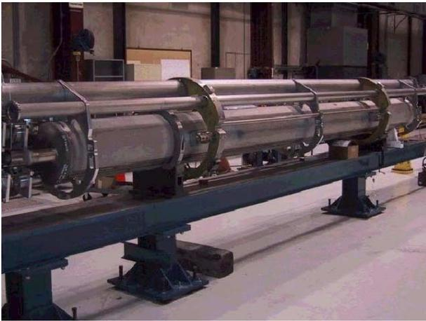
Figure 5: Prototype MQXB low- $\beta$  quadrupole ready for cryostating in Fermilab.
