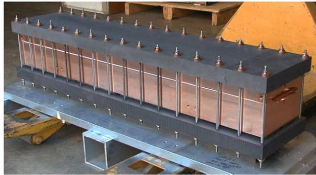
Figure 2 – RFQ clamping arrangement for GlidCop® to copper braze.
